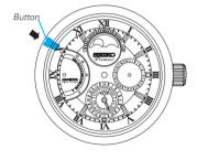
Press the button using an object with a long tapered tip such as a ballpoint pen.
