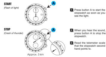
Please note that the stopwatch second hand moves in 1/5 second increments and does not always point exactly to the graduations of the telemeter scale. The telemeter scale can be used only when the measured time is less than 60 seconds.
