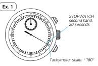
"180" (tachymeter scale figure) x 1 job = 180 jobs/hour
