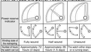
The watch employs a device to prevent overwinding of the mainspring. Once the mainspring is fully wound, the mainspring slips inside, disengaging the winding mechanism. When this happens, you can still turn the crown without damaging the watch, however, please refrain from excessive operation of the mainspring.
