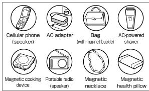
If the watch becomes magnetized and its accuracy deteriorates to an extent exceeding the specified rate under normal use, the watch may need to be demagnetized. In this case, you will be charged for demagnetization and accuracy readiustment even if it happens within the guarantee period.
