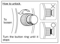
Turn the button ring counterclockwise (downward) to lower the slide cover gradually. Turn the button ring further until you can clearly see the guide line and the button ring can no longer be turned. Now the screw-lock type button is unlocked and can be operated.
